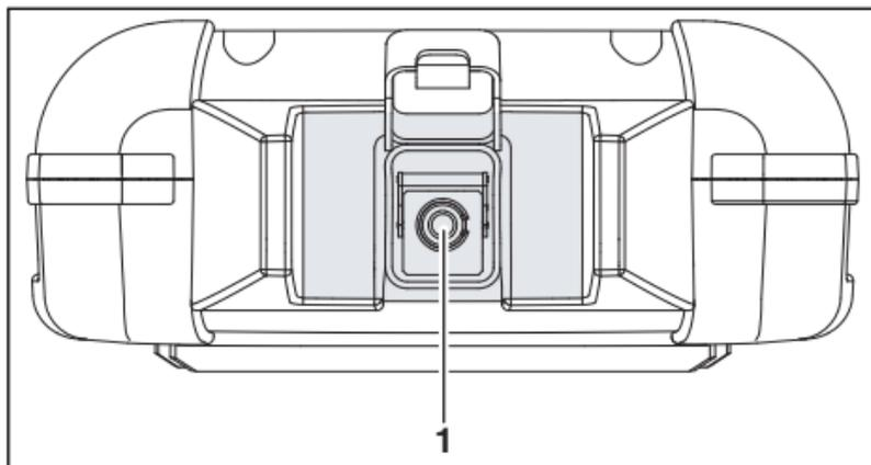
Fig. 2 OBS-550 connector panel
