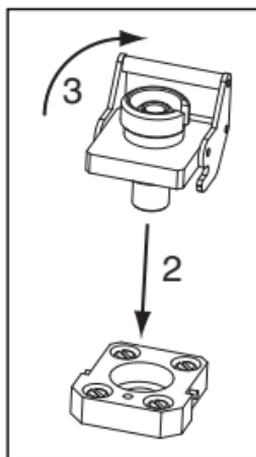
Fig. 5 Mounting the JAE test adapter
