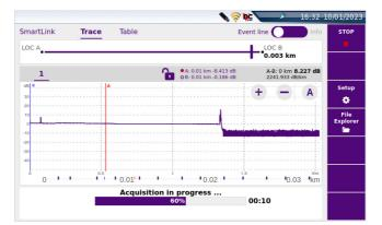
2 At the end of test, the OTDR trace(s) or SmartLink View is displayed.
