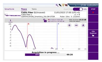
2 At the end of the test, the Smart Link view is displayed, with a pop up window indicating global test results (loss, length at each wavelength, and alarm status).
