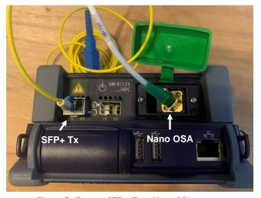
Figure 5: Connect SFP+ Tx to Nano OSA port
