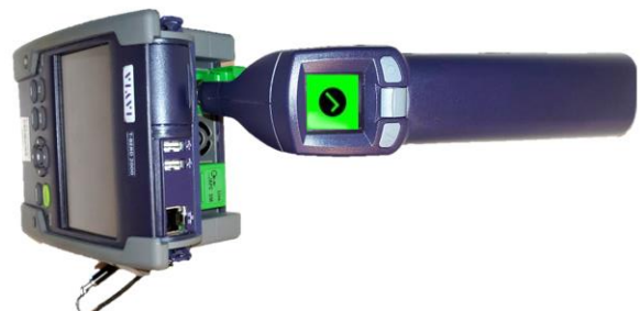
Figure 3: OTDR Port Inspection
