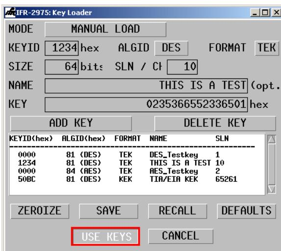
Figure 13.0 Loading keys using the Load Key function
