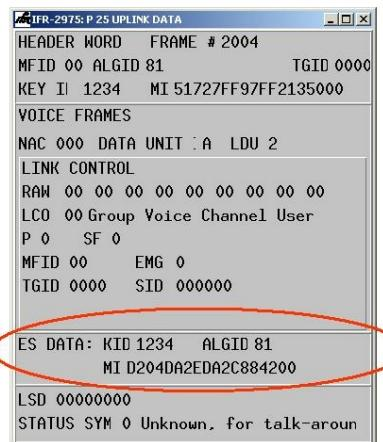
Figure 15.0 The P25 Uplink Data tile showing encryption parameter
