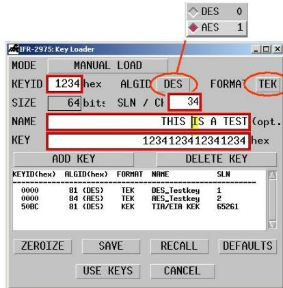
Figure 10.0 Setting up Encryption Key Parameters on the IFR 2975
