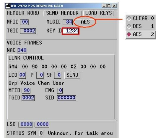
Figure 14.0 The P25 Down Link Data Tile showing AES and Key ID fields
