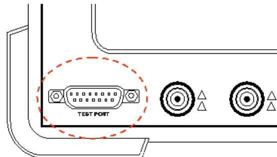
Figure 8.0 The IFR 2975 KFD Test Port on the front of the instrument
