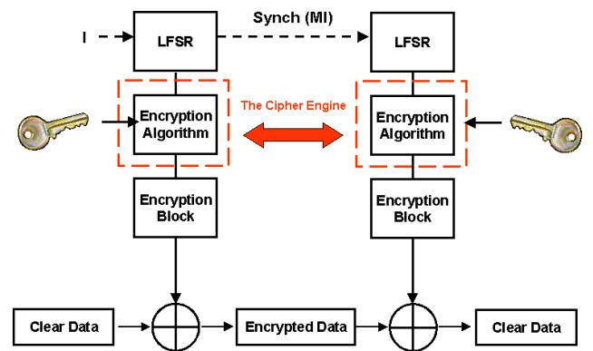
Figure 2.0 *Encryption System using Linear Feedback Shift Register*
