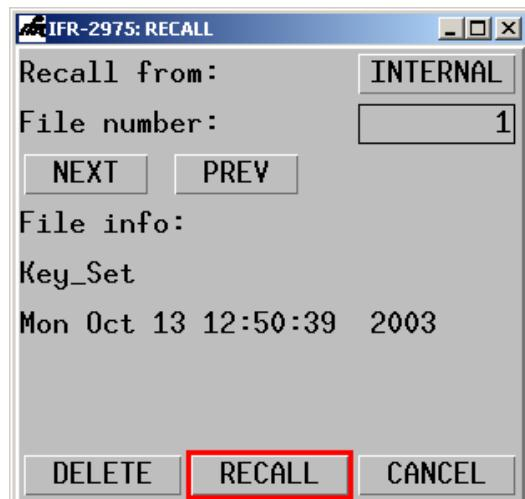
Figure 12.0 The Recall and Delete Key Set Function
