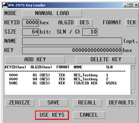
Figure 6.0 The IFR 2975's primary key loading screen
