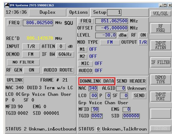
Figure 4.0 The IFR 2975 P25 Uplink and Downlink Data Tiles
