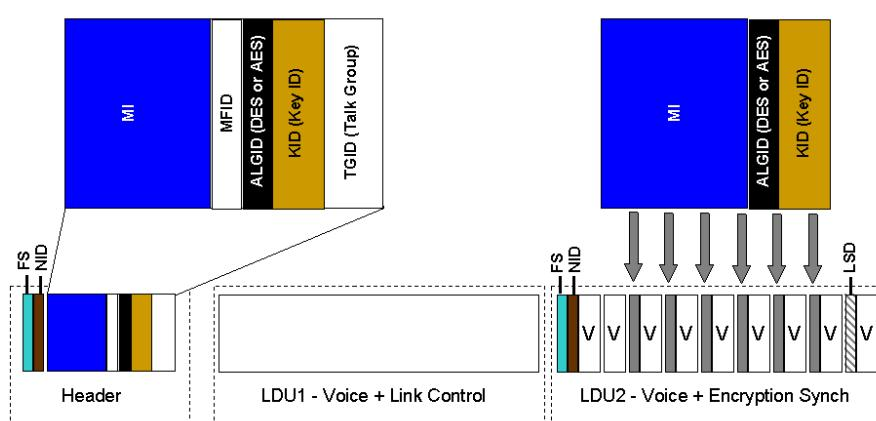
Figure 3.0 The P25 Super-frame and Mapping of the MI, ALGID and KID (Error Correction Coding not shown).
