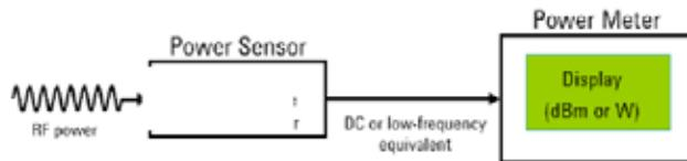
This above diagram shows the basic methodology of measuring high frequency power using the combination of power meter and power sensor. The power sensor converts high frequency power to a DC or low frequency signal that the power meter can measure and relate to an RF power level. The meter displays the direct signal as a power value in dB or watts.
