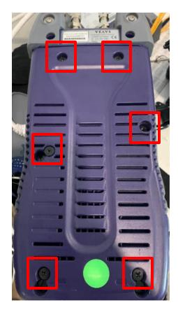
Remove OneExpert CATV cloth case and locate the 6 flat-head screws marked with the battery icon
