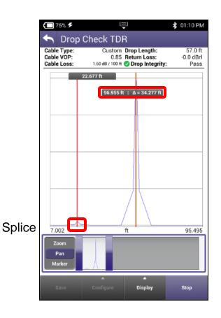
DROP CHECK and CABLE LENGTH tabs are identical tests. The DROP CHECK simply reminds the user to disconnect the other end of the drop.
