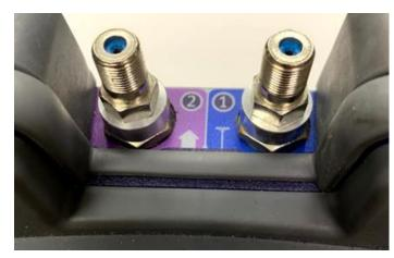
Start by removing the current F-81 adapter and collar (if present). If needed use a 7/16 wrench, turn the F connector counterclockwise until the adapter is completely out of the ONX RF port. Retain the collars if not replacing them with new ones.
