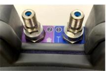
RF ports with collars between the F-81 barrelconnectors and ONX body
