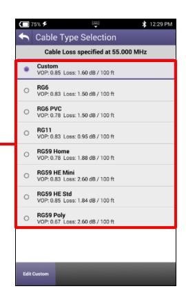
A TDR measures reflections based on time. Therefore the correct Velocity of Propagation for the cable to be tested must be chosen first.
