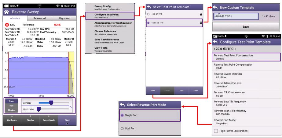
Reverse Sweep Configure Test Point Injection
