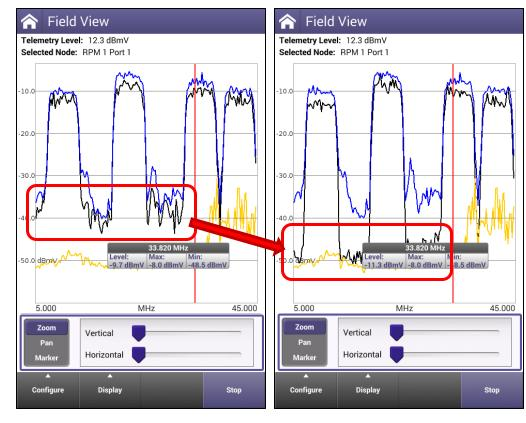
**Left:** Noise visible between the active upstream carriers **Right:** Noise source cleaned up reveals a much lower system noise floor
