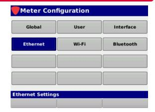
The **Ethernet** screen will be displayed as shown in the image to the right. This screen allows you to modify the Ethernet connection settings.
