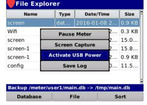
13. The power to the USB flash drive is activated and the drive is now mounted to the file system as shown in the image to the right. The 802 AWE is now capable of transferring files to and from the USB flash drive.
