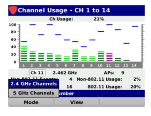
Select the Mode softkey to toggle the display mode between 2.4 GHz and 5 GHz channels.
