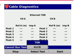
ALCD – This test is performed over an active cable that uses a passive measurement method to estimate the cable length present during an active link.
