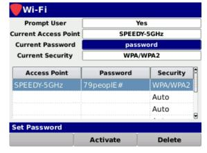
Press the **Enter** button and the **Virtual Keyboard** will be displayed as shown in the image to the right. Use the **Virtual Keyboard** to enter the password of the Wi-Fi network.
