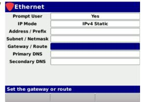
Press the **Enter** button and the **Virtual Keyboard** will be displayed as shown in the image to the right. Use the **Virtual Keyboard** to enter the gateway address in the ###.###.### format.
