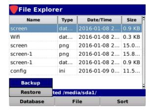
The Message Bar will indicate a successful backup to the flash drive by displaying the text "-> /media/sda1/main.db" as shown in the image to the right.
