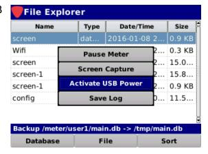
4. The power to the USB flash drive is activated and the drive is now mounted to the file system as shown in the image to the right. The 802 AWE is now capable of transferring files to and from the USB flash drive.
