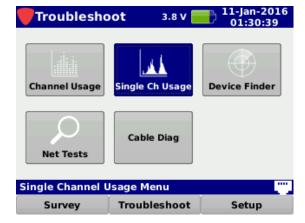
The **Single Channel Usage** screen will be displayed as shown in the image to the right. Each of these screens allows you to select a single 2.4 GHz or 5 GHz wireless channel.
