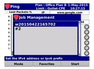
If you don't want to save the test to the open job, select **No** and you will be prompted to enter a file name using the **Virtual Keyboard**. It will then be saved to the internal memory of the 802 AWE.
