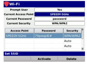
Press the **Enter** button and the **Virtual Keyboard** will be displayed as shown in the image to the right. Use the **Virtual Keyboard** to enter the name of the access point.
