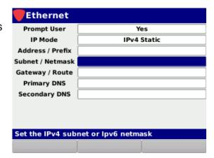
Press the **Enter** button and the **Virtual Keyboard** will be displayed as shown in the image to the right. Use the **Virtual Keyboard** to enter the subnet address in the ###.###.### format.
