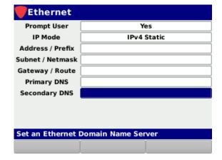
Press the **Enter** button and the **Virtual Keyboard** will be displayed as shown in the image to the right. Use the **Virtual Keyboard** to enter the secondary DNS address in the ###.###.### format.
