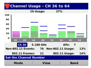
space on the graph will be occupied by part of the 802.11 percentage of utilization. In this case, the non-802.11 percentage of utilization acts as a noise floor that squeezes out the desired 802.11 percentage of utilization.
