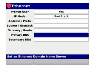
Press the **Enter** button and the **Virtual Keyboard** will be displayed as shown in the image to the right. Use the **Virtual Keyboard** to enter the primary DNS address in the ###.###.### format.
