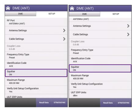
Figure 6-15 DME Unique Setup Parameters
