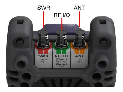
Figure 2-3 I/O Connectors
