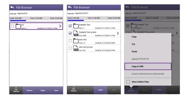
Figure 9-23 Guided Test Copy to USB
