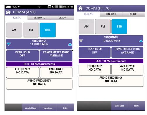
Figure 7-9 COMM High Frequency (HF) Single Side Band (SSB) Receive
