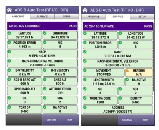
Figure 4-22 Completed ADS-B Auto Test Screens
