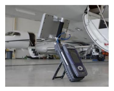
Figure 3-2 Over-the-Air Test Set-Up
