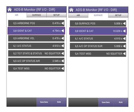
Figure 4-23 ADS-B Monitor Air and Surface
