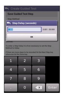
Figure 9-9 Guided Test Step Method - Delay
