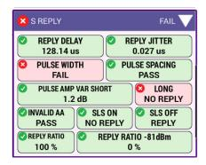
Figure 4-8 Example XPDR Mode S Reply Fail
