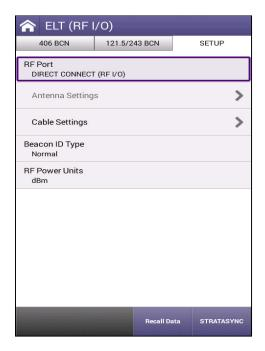
Figure 8-2 ELT (Emergency Location Transmitter) Unique Setup
