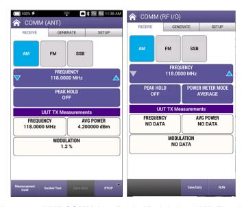
Figure 7-5 VHF COMM Amplitude Modulation (AM) Receive
