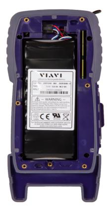
Figure F-4 Replacement Battery / Location
