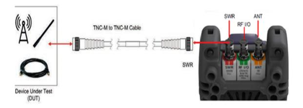
Figure 10-9 DTF Test Setup
