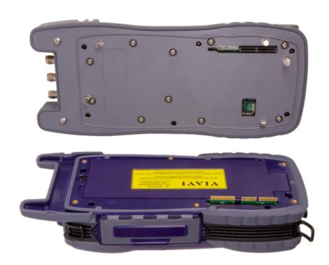
Figure 12-3 Battery Cover Removal
