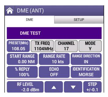
Figure 6-16 DME Preset Frequency Entry
