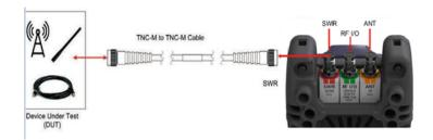
Figure 10-7 Perform VSWR Test Setup
