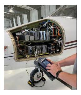
Figure 3-5 Direct to UUT Test Setup
