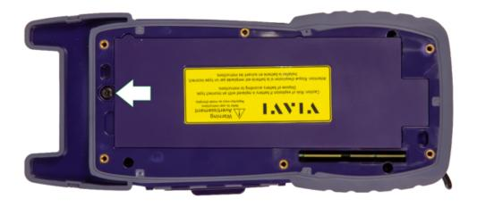
Figure 12-4 Battery Cover Screw Removal
