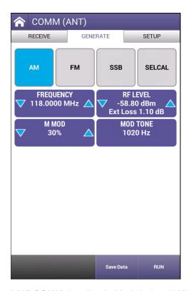
Figure 7-6 VHF COMM Amplitude Modulation (AM) Generate
