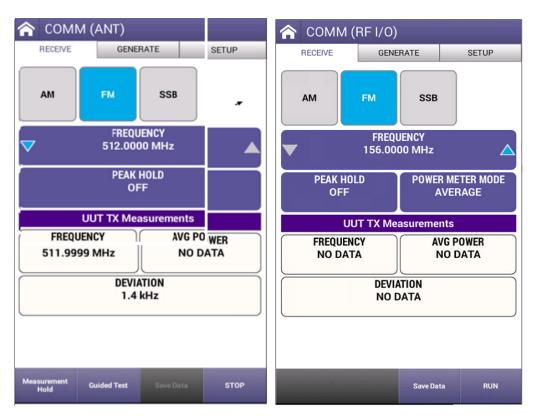
Figure 7-7 VHF COMM Frequency Modulation (FM) Receive
