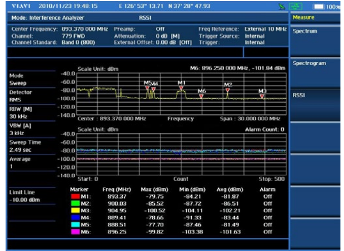
Interference analysis test — RSSI
