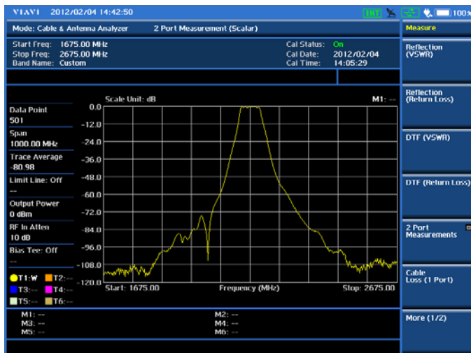
Cable and antenna test — 2-port Measurement
