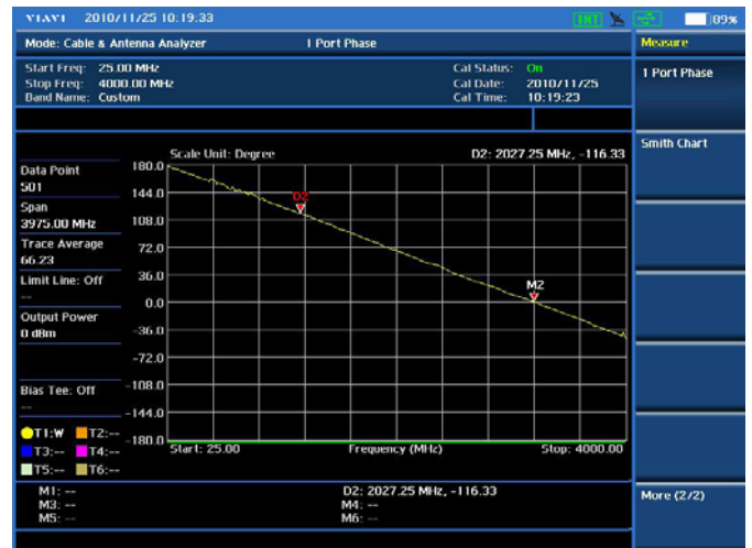
Cable and antenna test — 1-Port Phase
