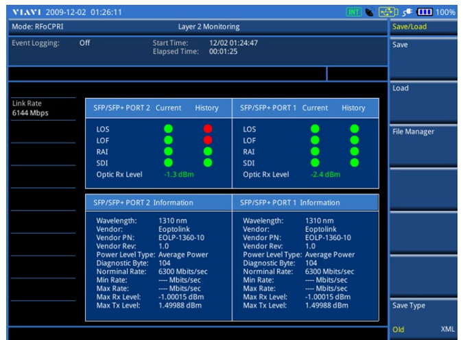
RFoCPRI — Layer-2 Monitoring
