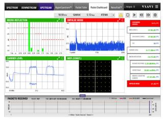
Figure 11. VSE-1100 Packet Dashboard display with impulse noise causing code Word errors
