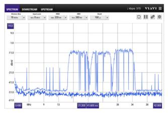
Figure 4. Swept spectrum analyzer with impulse noise and DOCSIS carrier
