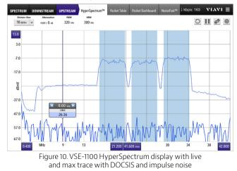
Figure 10 shows the first displayed live max trace from a VIAVI Solutions VSE-1100 spectrum analyzer in HyperSpectrum mode. The instrument captures all the DOCSIS channels clearly and the impulse noise in less than 1 sec.
