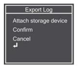
The export operation takes several minutes to complete. While the operation is in progress, the Busy LED on the CleanBlastPRO lights yellow. When the operation is completed, the Busy LED turns off and the Ready LED lights green.
