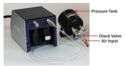
**Note:** The air filter canisters of the CleanBlastPRO can act as a small volume air tank. Using a check valve before the air input to the CleanBlastPRO exactly as shown in Figure 4-3 can be helpful if the air supply might be briefly (less than one second) impacted or if the supply runs are poor.
