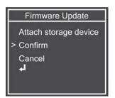
The firmware update takes several minutes to complete. While the update is in progress, the Busy LED on the CleanBlastPRO lights yellow. When the update is completed, the CleanBlastPRO automatically restarts (powers off and then powers on).
