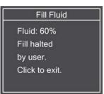
**Note:** If the solvent runs out before the tank is full, auto fill will automatically stop. Observe the message that appears on the LCD screen.
