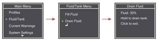
Step 6 Press and hold the dial until the fluid begins to drain from the handset into the container, and then release the dial. Observe the message that appears on the LCD screen.
