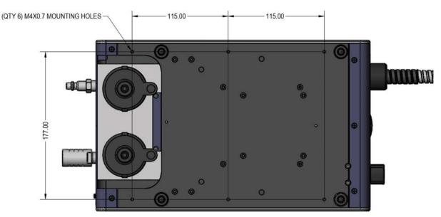
Figure 2-7: CleanBlastPRO underside - threaded (M4X0.7-6H) mounting holes
