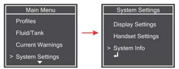
c. On the **System Info** menu, scroll to **Filter Age**, and then hold down the dial to reset the value to 0.
