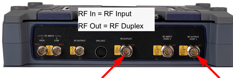
Figure 6-4 RF Duplex/RF Input Two Port Duplex Test Setup
