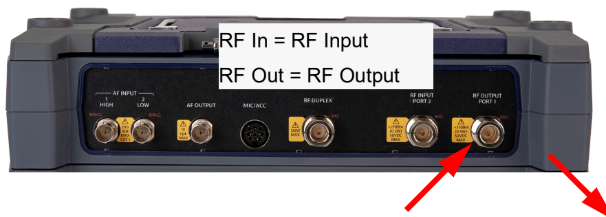
Figure 6-2 RF Output/RF Input Two Port Duplex Test Setup
