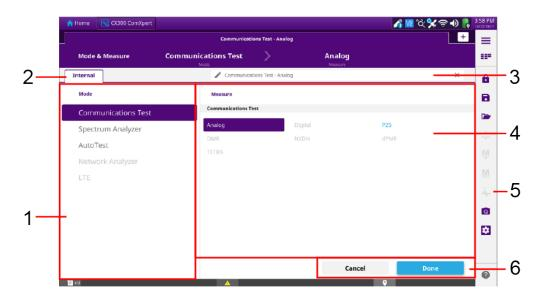
Figure 5-1 Test Home Screen - Layout Diagram
