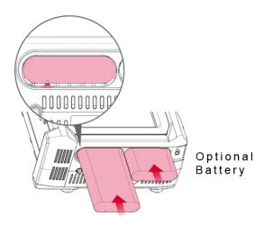
Figure 8-2 Battery Installation Diagram
