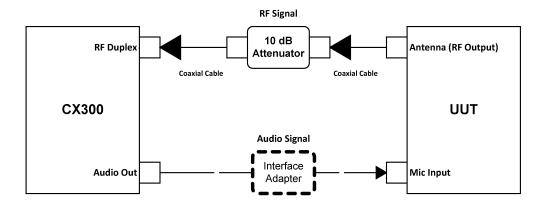
Figure 6-7 Digital Receiver Test Setup Diagram
