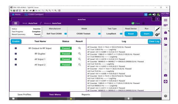
Figure 6-5 Self Test Screen (Example)
