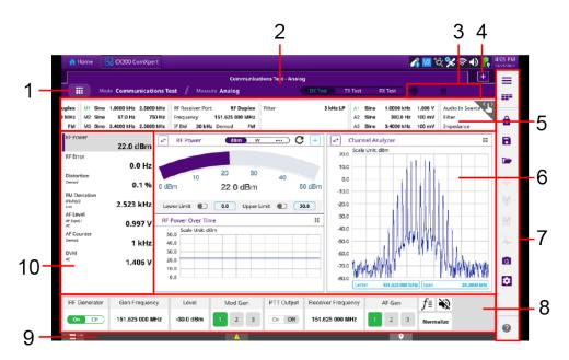
Figure 5-2 Example of Test and Measurement Main Screen
