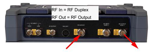
Figure 6-3 RF Output/RF Duplex Two Port Duplex Test Setup
