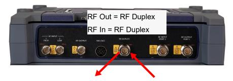
Figure 6-1 One Port Duplex Test Setup
