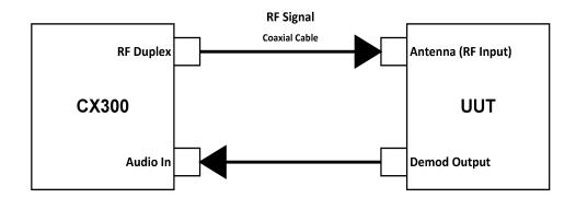
Figure 6-9 Channel Power Measurements Setup Diagram
