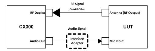
Figure 6-6 Digital Transmitter Test Setup Diagram
