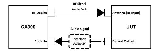
Figure 6-8 Receiver Test Setup Diagram
