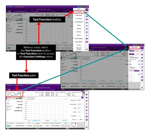
Figure 5-18 Test Function pane & Test Function Settings
