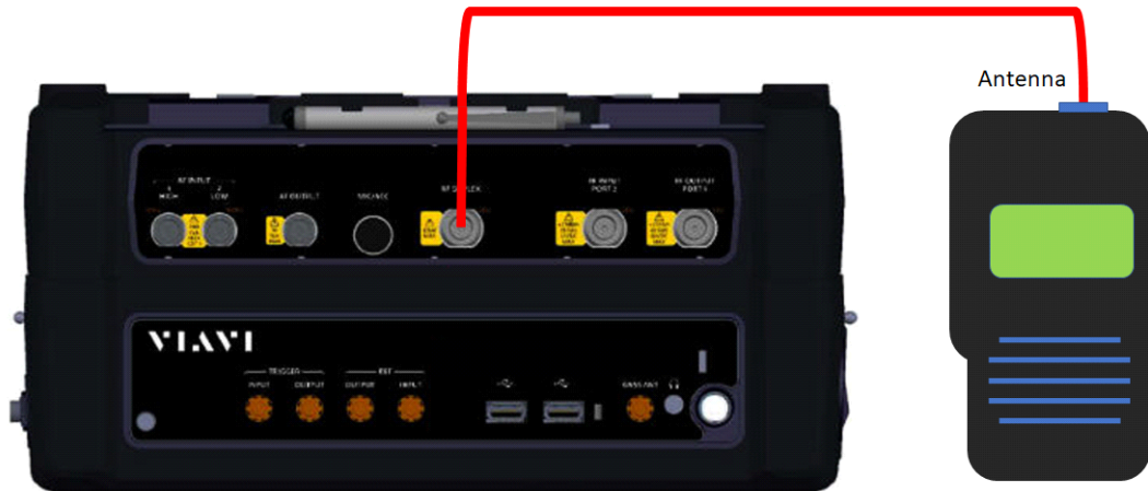
Figure 3-1 P25 Transceiver Test Setup Diagram
