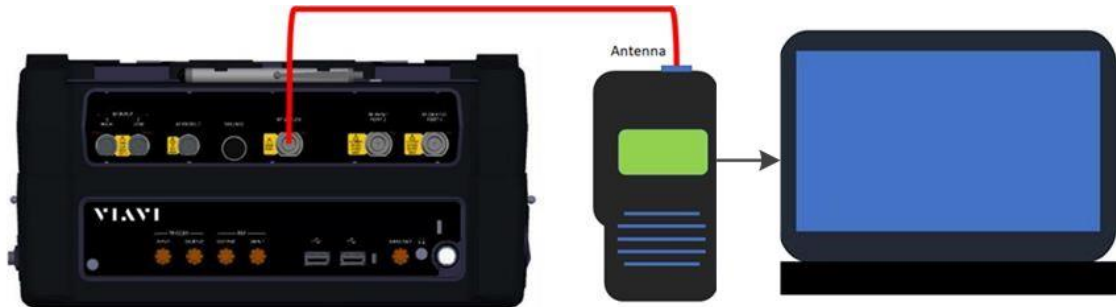
Figure 3-2 P25 Receiver Sensitivity Test Setup Diagram
