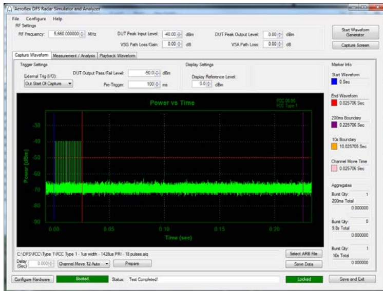
Figure 4. Channel Closing Time/Channel Move Time (zoom)
