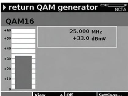
The Return QAM Generator enables operators to test and prove upstream network performance.
