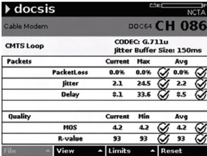
VoIPCheck displays packet loss, jitter and delay as well as MOS and R-values.
