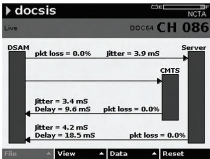
VoIPCheck is a voice quality verification test that runs over the DSAM's cable modem DOCSIS connection. It allows for segmentation between HFC and IP issues by showing on which side of the CMTS data impairments are present.
