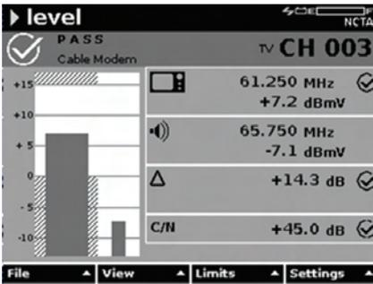
Level mode on an analog channel displays video and audio signal levels and their delta value. Carrier-to-Noise (C/N) ratio is also displayed.
