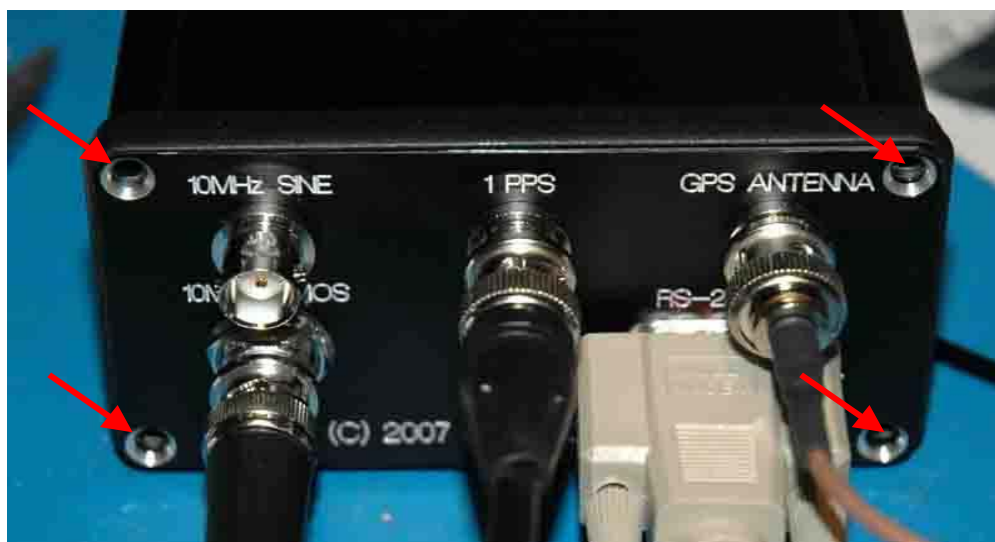
Figure 4.2 Fury faceplate removal.
