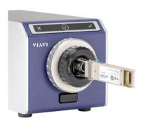
Technicians can leverage the FVAM-2000's built-in intelligence to streamline the fiber inspection process. By automating setup, tip configuration, testing, and data storage, it replaces the need for outdated manual devices. Simply attach the desired adapter and let the microscope handle the rest:
