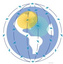
A 'warm start' is just a power cycle of the GPS Receiver. This can be helpful in some situations, but there are other situations where a 'cold start' might be required. A 'cold start' involves a reset of the GPS Receiver's memory so that it 'forgets' any previous information and will re-acquire GPS satellites as a new event. A 'cold start' typically takes longer for the GPS Receiver to lock.
