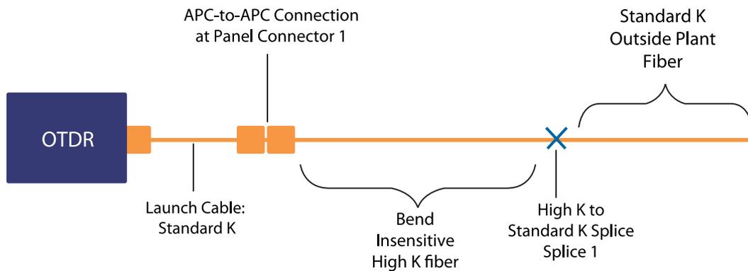
Figure 1. Test setup for forward measurement of Splice 1 using a standard K fiber
