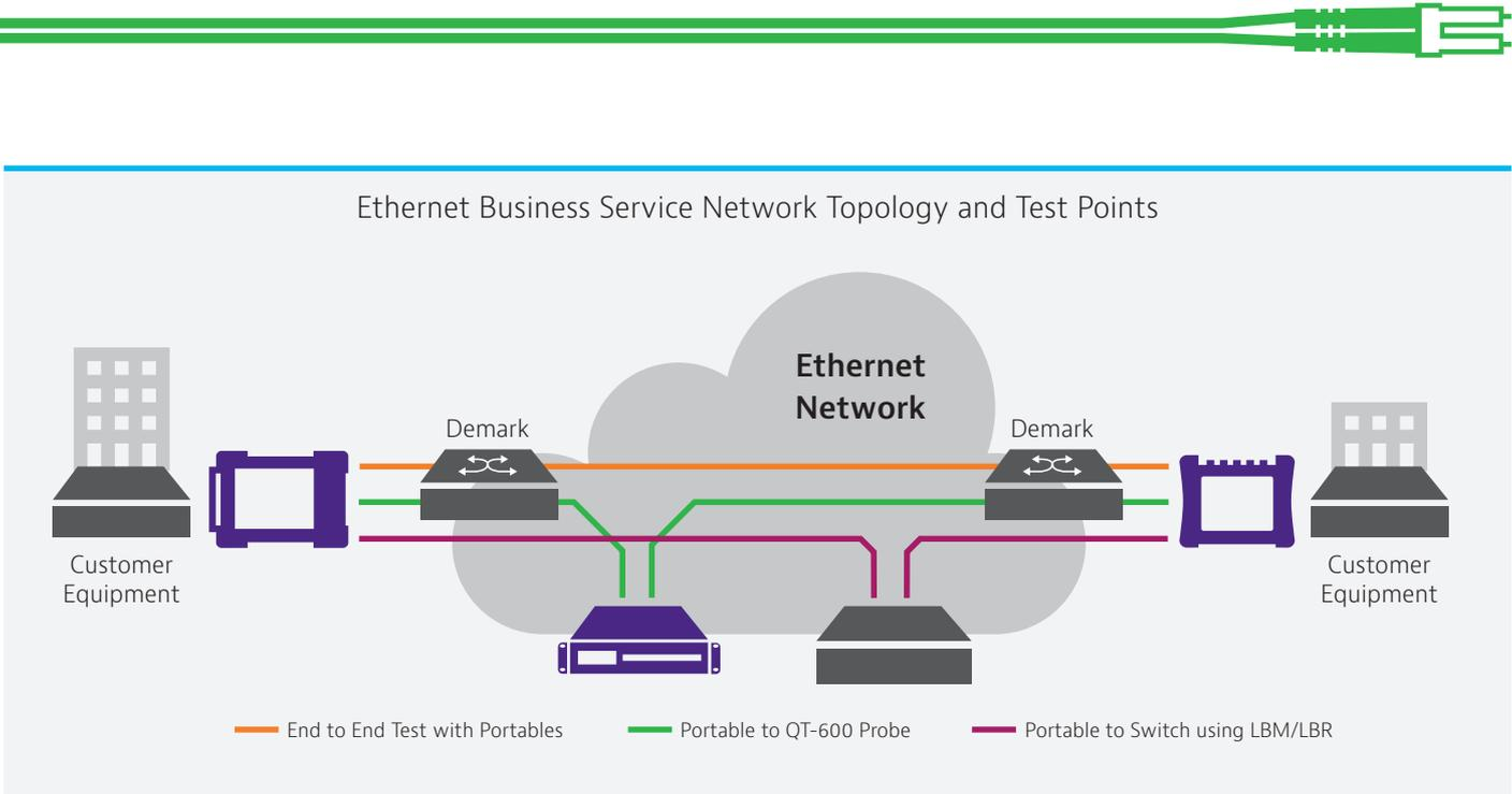
The diagram above shows the “local” T-BERD/MTS represented on the left side and the “remote” T-BERD/MTS on the right. The most common service activation use case is a loop-back of the remote device and in this case, the device will be the remote T-BERD/MTS.
