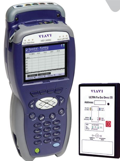
A two-ended test provides accurate fault identification for wideband services
