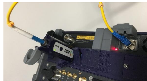
Figure 5: Test fibers connected to the OTDR Port and MP60 installed on OneAdvisor-800
