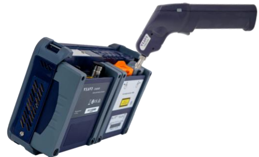
Figure 3: OTDR Port Inspection
