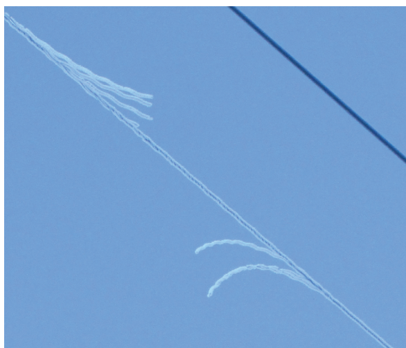
Picture 1b: Broken strength members
