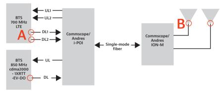
Figure 1. Signal level measurement points
