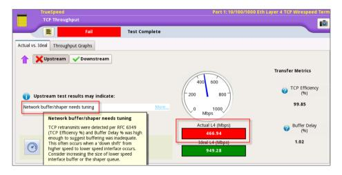
Fusion TrueSpeed VNF's integrated, hardware-based traffic shaping function allows the provider to demonstrate the difference in performance when traffic shaping is enabled, and provides definitive proof that the WAN can properly transport end customer TCP traffic.
