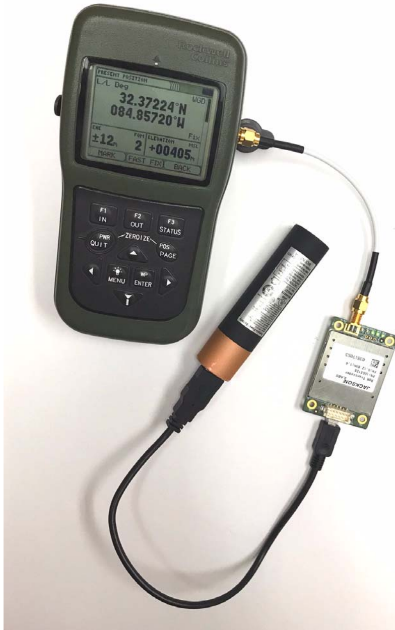
Figure 2.2 DAGR Target Receiver with battery-powered RSR GNSS Transcoder™
