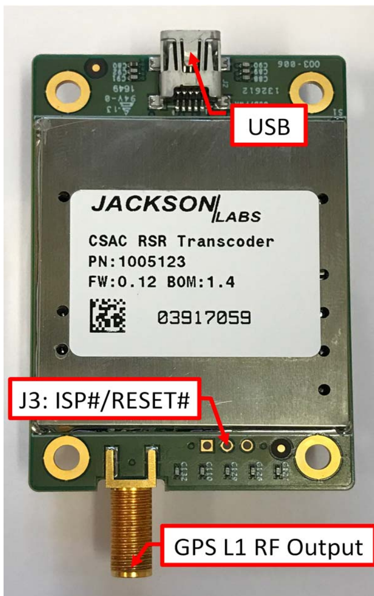
Figure 7.1 Location of ISP and Reset header J3
