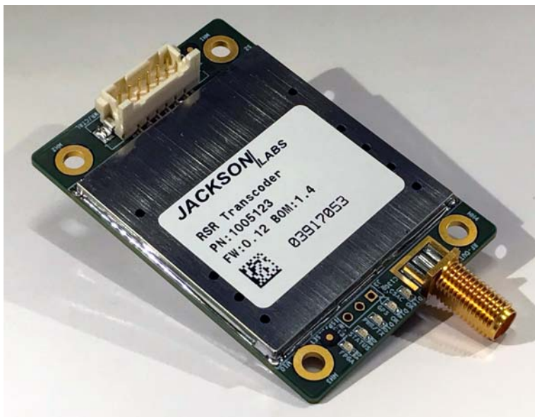
Figure 1.1 RSR GNSS Transcoder™ PCB module (TCXO version)
