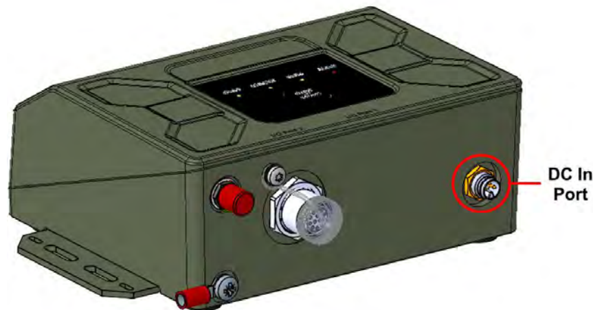
Figure 5 DC In port location on enclosure
