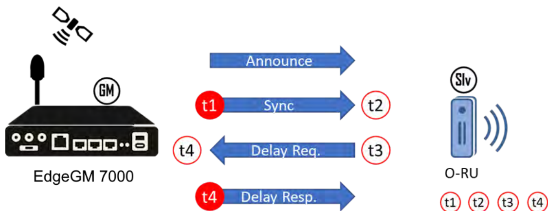
Figure 4-107: Basic working principle of IEEE 1588v2
