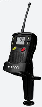
Seeker D has a wide sensitivity range (2–2000  $\mu$ V/m). In the NAV band, the Seeker D detects the proprietary signal from the CT-4 or R-PHY unit and scales them to be similar to leakage readings taken from an analog carrier. Consequently, readings taken from the Seeker meter and Seeker D meter produce similar results in the aeronautical band.
