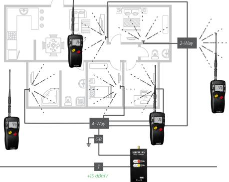
Using the Seeker HL with its source transmitter allows the technician to detect leakage levels at an otherwise unheard of sensitivity down to 0.1  $\mu$ V/m. The user may set the output level to 60 dBmV for home certification, but also has the option to reduce the level to 40 dBmV should the subscriber network prove to be too porous for pinpointing the location of a leak at the higher transmit level.
