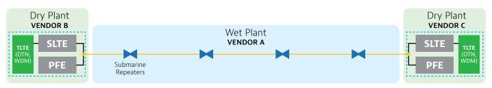
SLTE Submarine Line terminal Equipment · PFE Power Feed Equipment · TLTE Terrestrial Line Terminal Equipment
