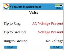
Indicates AC and DC voltages via the Volt/Ohm mode
