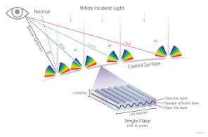
Figure 4. Diffractive theory diagram
