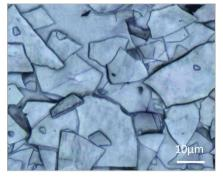
Figure 2. Microscopic image of Bright Silver showing flake's smooth surface.
