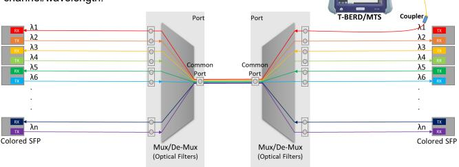
Figure 4: Connecting to the Fiber Under Test
