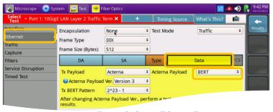
Figure 8: Setup, Ethernet/Data
