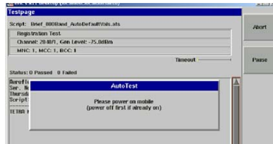
Fig 3: Registration test - operator prompted to turn on the UUT
