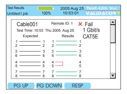
Figure 4.3 Test Results Short on Pair 4 and 5
