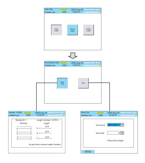
Figure 5.3 Phone Manual Test Flowchart
