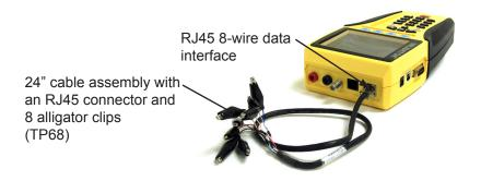
Figure 2. TP68 Connected to Validator
