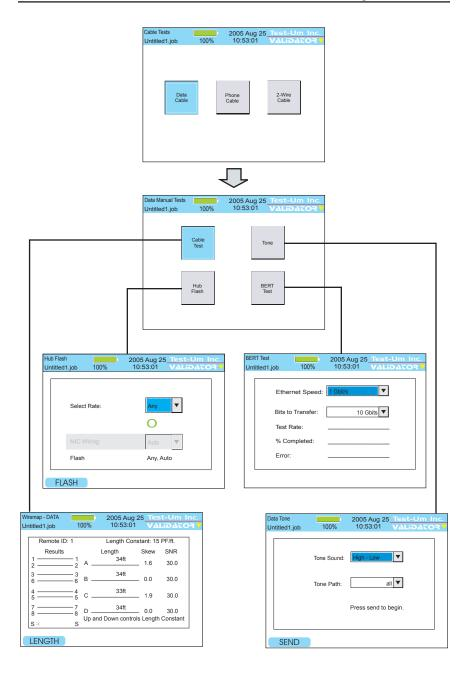
Figure 5.2 Data Manual Test Flowchart
