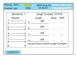
Figure 5.7 Testing Cable Length
