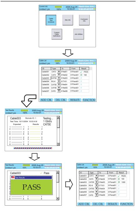
Figure 4.1 Auto Test Flowchart
