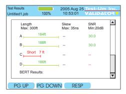
Figure 4.4 Page down to Display Distance to Short
