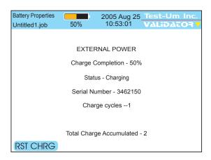
Figure 2.3 Unit Operating on External Power
