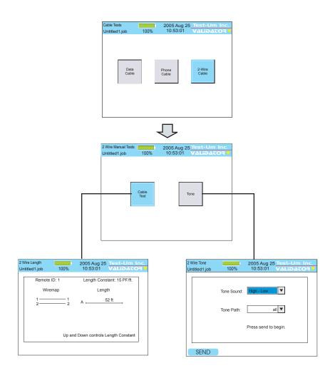
Figure 5.4 Two Wire Manual Test Flowchart
