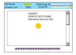
Figure 4.7 Cable Test without Remote
