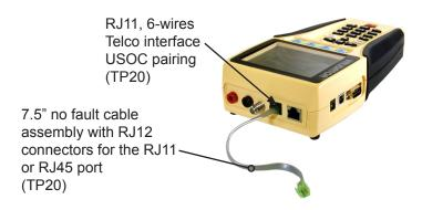
Figure 3. TP20 Connected to Validator
