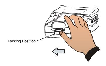
Figure 11. Battery Locking Position
