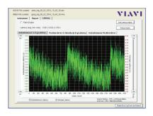
The ADS-B INTEGRITY™ software application, supports Supplemental Type Certification (STC) and post approval testing for ADS-B Out equipment installations. For accuracy and integrity performance test, the software controls the VIAVI IFR6000 or IFR6015 Transponder Test Set. An additional positional accuracy test is accomplished with the VIAVI GPSG-1000 Positional Simulator.
