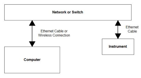
Another method of connection is that the computer is connected to a network or a switch, and the instrument is also connected to the network or switch. Again, a common Ethernet cable can be used. to connect the instrument to the network.
