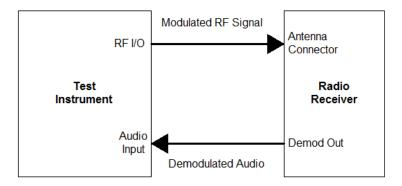
The RF I/O connector of the test instrument must be connected to the antenna connector of the radio receiver. If an Over The Air (OTA) connection is required, connect the instrument RF I/O connector to an antenna instead of making the direct connection pictured above.
