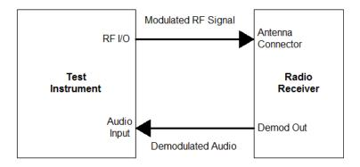
To run find\_sinad, the RF I/O connector of the test instrument must be connected to the antenna connector of the radio receiver.
