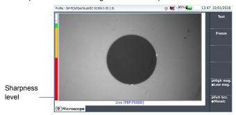
Use the **Focus Control** button onto the P5000i scope (see Figure 21 on page 50) to adjust the image quality and sharpness.
