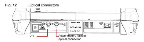
The type of optical connector used for the power meter is UPP (Universal Push Pull), which is compatible with all diameter 2.5 mm connectors (FC, SC, ST, DIN, E2000, etc.)
