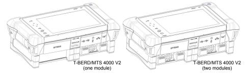
Fig. 2 4000 V2 Platform: Front view TFT 9" Color Touchscreen
