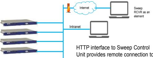
Unit provides remote connection to easily manage configurations remotely
