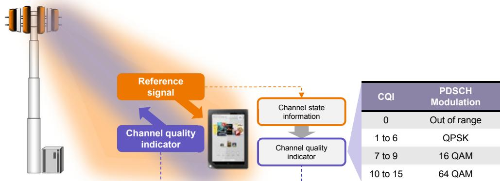
Figure 7. RF environment assessment (via reference signals) and CQI
