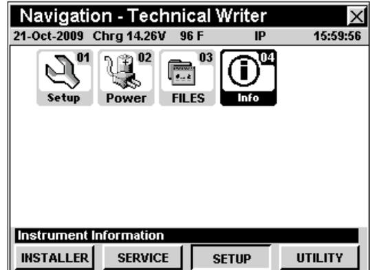
Use the **▲ ▼** buttons to select the **RF Option Info** field. If the FDR Option is installed, the widow will display the text **FDR : YES**.
