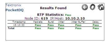
The RTP Statistics results include 5 additional results families, each with pass/fail limits. Each of these categories provides additional information accessible by selecting the pass/fail parameter link.
