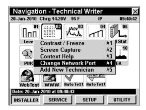
Use the buttons to highlight the **External RJ45**, **Internal Modem**, or **Wi-Fi** network port, and then press the button.
