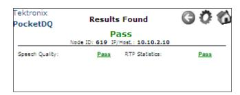
The RTP Reflector top-level results display shows two results families: Speech Quality and RTP Statistics. Drilling down by selecting the pass/fail parameter provides the following information.
