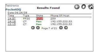
Search results are grouped by date, as seen in the above results display. The "State" column provides overall Pass or Fail information. The "Phone/IP" column displays the phone number or IP address of termination.
