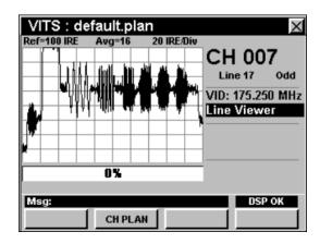
By looking at the spectrum of the multiburst signal, it is possible to measure in-channel response by comparing the maximum variation in the magnitudes of each discrete burst frequency to the FCC limit.
