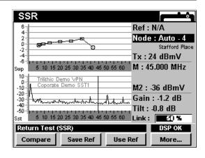
To change the node, use the buttons to highlight **Node** and use the buttons to increment the value up and down.
