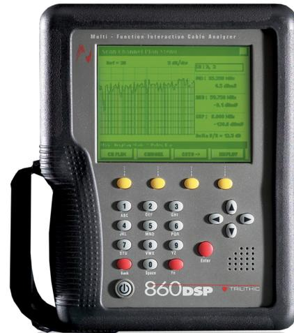
The 860 DSP™ provides all of the testing power needed to insure HFC networks operate to the highest standards. This includes balancing the distribution system, maintaining analog and digital signal quality, controlling return path ingress, and much more. Several options equip the 860 DSP cable analyzer for a variety of roles, and all configurations feature an attractive price.
