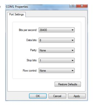
3. Connect to the 860 DSPh by selecting **OK** and then press **ENTER**. The 860 DSPh prompt will be displayed as follows;
