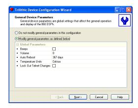
**Auto Reboot:** Enter the number of days the unit will operate for before automatically rebooting. (Enter 0 to turn off automatic rebooting.)
