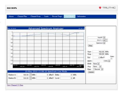
displacement represents signal strength. The horizontal axis represents a range of frequencies.
