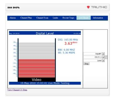
Select the <u>View Channel # Data</u> link to view the channel details as shown in the Alarms Display section.
