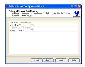
desired for periodic maintenance, but is not necessary (and probably should not be performed) each time a device is configured. This option is only available if you have selected Add Selected Items and Delete All Other Items on the Packet Mode Transfer screen shown in the previous step.
