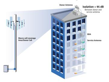
In this case, the BDA gain was 80 dB, so an isolation of 95 dB was required.
